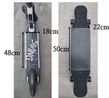
Fig. 10 Comparison of actual electric kickboard and the designed skateboard deck size
